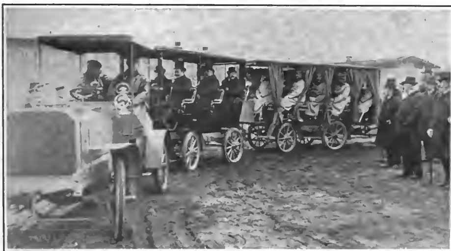
DEMONSTRATION TO SHOW HOW EACH CAR FOLLOWS IN TRACKS OF LEADER IN TURNING.
